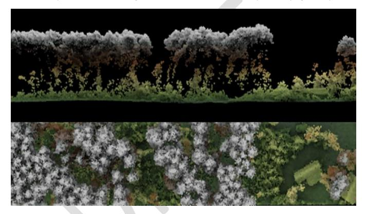
Figure 5: Lidar point cloud in an area of Cass County, Minnesota, collected in October 2017 (full leaf on, peak fall color). Top image depicts a cross section, colorized by height, and the bottom image is the overhead view of the same location.
