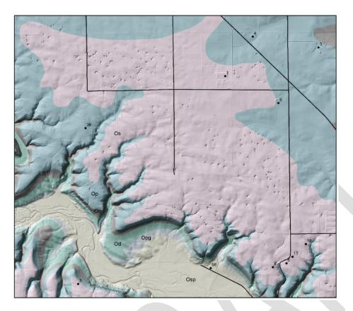
Figure 3: Portion of Olmsted County with geological mapping superimposed on a lidar-based digital elevation model (DEM). Sinkholes are apparent as small pits, and preferentially occur within the Stewartville Formation, labelled with "Os". Black dots show water wells with depth to bedrock in feet.
